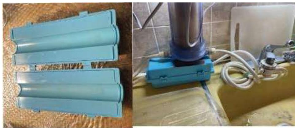
Left image is open position of 2 pieces magnets placed in repelling position forms as a housing to water pipe with hinges once put 2 pieces put together.
